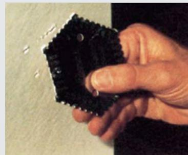
Surfaces should be abrasive blast cleaned to minimum Sa 2.5 BS EN ISO 8501-1:2001 with a surface profile not exceeding 100 microns. Any spent abrasive should be removed by vacuum, clean compressed air or brush.
